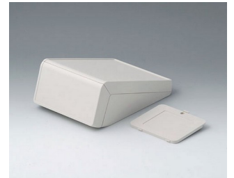
B4054337 UNITEC S, 0,6/1,4 ABS (UL 94 HB) gris blanc RAL 9002 125x177x69mm IP 40
