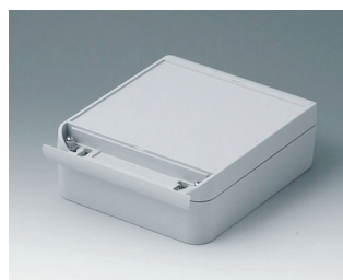
C6015181 SMART-BOX 150 LARGE ASA+PC-FR (UL 94 V-0) gris clair RAL 7035 180x150x60mm IP 66
