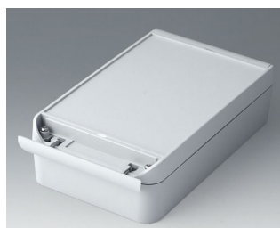
C6013221 SMART-BOX 130 LARGE ASA+PC-FR (UL 94 V-0) gris clair RAL 7035 220x130x60mm IP 66
