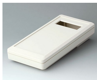
A9075217 DATEC-MOBIL-BOX L, Vers. II ABS (UL 94 HB) gris blanc RAL 9002 252x121x50mm IP 65 opt.
