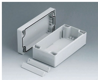
C2008161 ROBUST-BOX 80 LARGE, Vers. I ABS (UL 94 HB) gris clair RAL 7035 160x80x60mm IP 66
