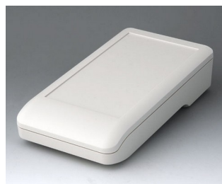
A9007117 DATEC-COMPACT L ASA+PC (UL 94 V-0) gris blanc RAL 9002 206x110x47mm IP 41
