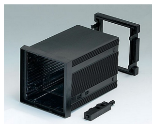
B6023031 BOITIER ENCASTRABLE TYPE A PPO (UL 94 V-0) noir RAL 9005 72x72x100mm
