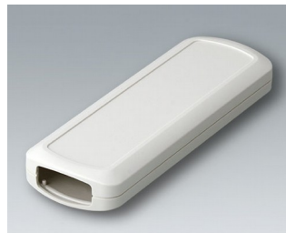
B2834107 CONNECT ASA+PC-FR (UL 94 V-0) gris blanc RAL 9002 156x54x22mm IP 40
