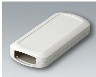
B2833107 CONNECT ASA+PC-FR (UL 94 V-0) gris blanc RAL 9002 116x54x22mm IP 40
