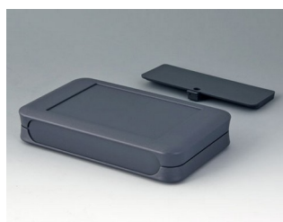
A9053118 SOFT-CASE XL ABS (UL 94 HB) lava 92x150x28mm IP 40
