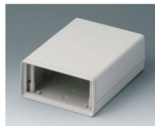
A9413340 BOITIER COQUILLES O 190, Vers. I ABS (UL 94 HB) gris blanc RAL 9002 138x190x68mm
