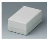
A9406341 BOITIER COQUILLES G 110, Vers. I ABS (UL 94 HB) gris blanc RAL 9002 72x114x45mm IP 65 opt.
