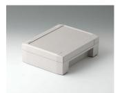
C8014182 SOLID-BOX 145 PC+ABS (UL 94 V-0) gris clair RAL 7035 180x145x60mm IP 66, IP 67, IK 08
