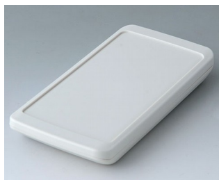
B5403307 SLIM-CASE M, Vers. III ASA+PC-FR (UL 94 V-0) gris blanc RAL 9002 148x74x19mm IP 65 opt., IP 40
