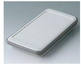
B5403317 SLIM-CASE M, Vers. VI ASA+PC (UL 94 V-0) gris blanc RAL 9002 148x74x22mm IP 54
