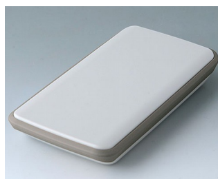
B5403117 SLIM-CASE M, Vers. IV ASA+PC-FR (UL 94 V-0) gris blanc RAL 9002 148x74x22mm IP 54
