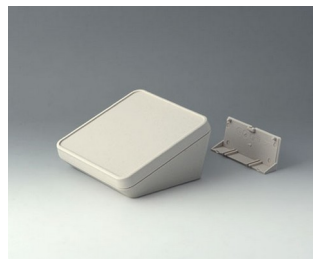
B4414207 PROTEC 140, Vers. II ASA+PC (UL 94 V-0) gris blanc RAL 9002 140x140x76mm IP 65 opt.
