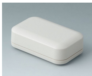
A9403107 EVOTEC 80, Vers. I ASA+PC-FR (UL 94 V-0) gris blanc RAL 9002 80x50x26mm IP 65 opt., IP 40
