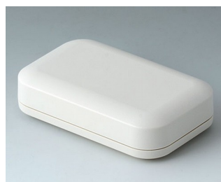
A9421107 EVOTEC 100, Vers. I ASA+PC-FR (UL 94 V-0) gris blanc RAL 9002 100x62x26mm IP 65 opt., IP 40
