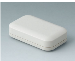
A9401107 EVOTEC 80, Vers. I ASA+PC (UL 94 V-0) gris blanc RAL 9002 80x50x22mm IP 65 opt., IP 40
