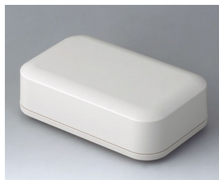
A9443107 EVOTEC 150, Vers. I ASA+PC-FR (UL 94 V-0) gris blanc RAL 9002 150x93x45mm IP 65 opt., IP 40
