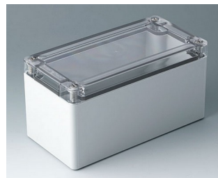
C7016025 IN-BOX PC gris clair RAL 7035 162x82x85mm IP 66, IP 67, IK 08
