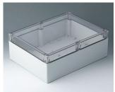
C7030114 IN-BOX ABS/PC (UL 94 HB) gris clair RAL 7035 302x232x110mm IP 66, IP 67, IK 07
