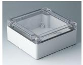
C7013034 IN-BOX ABS/PC (UL 94 HB) gris clair RAL 7035 124x122x55mm IP 66, IP 67, IK 07
