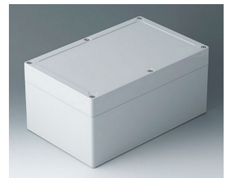
C7025091 IN-BOX ABS (UL 94 HB) gris clair RAL 7035 252x162x120mm IP 66, IP 67, IK 07
