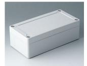
C7016011 IN-BOX ABS (UL 94 HB) gris clair RAL 7035 162x82x55mm IP 66, IP 67, IK 07
