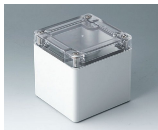
C7008025 IN-BOX PC gris clair RAL 7035 84x82x85mm IP 66, IP 67, IK 08
