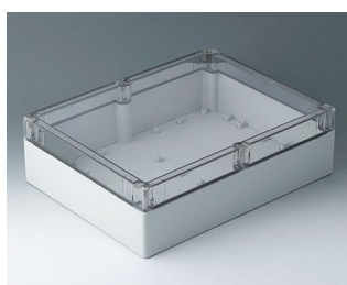
C7030104 IN-BOX ABS/PC (UL 94 HB) gris clair RAL 7035 302x232x90mm IP 66, IP 67, IK 07
