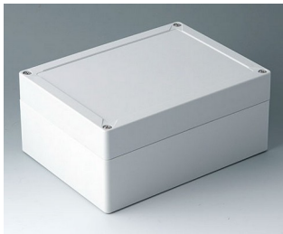
C7021072 IN-BOX PC gris clair RAL 7035 202x152x90mm IP 66, IP 67, IK 08
