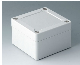
C7008012 IN-BOX PC gris clair RAL 7035 84x82x55mm IP 66, IP 67, IK 08
