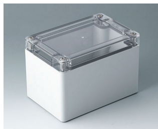
C7012025 IN-BOX PC gris clair RAL 7035 122x82x85mm IP 66, IP 67, IK 08
