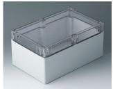
C7025094 IN-BOX ABS/PC (UL 94 HB) gris clair RAL 7035 252x162x120mm IP 66, IP 67, IK 07
